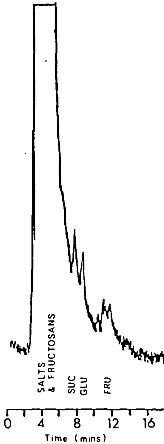
FIGURE 1: Chromatographic Profile of Neutral Sugar Extract of Developing Wheat Grain. (Refractometer attenuation x 1) 20ul injection from 8ml of a neutralised PCA extract of 100mg wet weight of endosperm tissue. Approximate amounts of Sucrose, Glucose and Fructose were 5.7 nmoles, 0.9 nmoles and 3.8 nmoles respectively.
